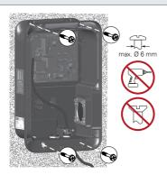
Fasten lower part of housing with 4 suitable screws
